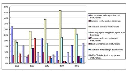
Fig. 10. Shares of various mechanical interruptions among excavator mechanical interruptions
