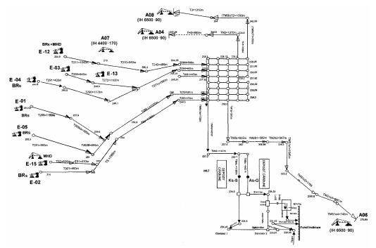
Fig. 2. Lignite open pits technological flow
